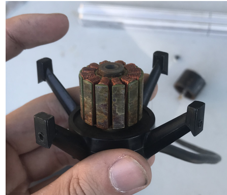
Figure 3. One of Charybdis' Older T200 Thruster Stators
